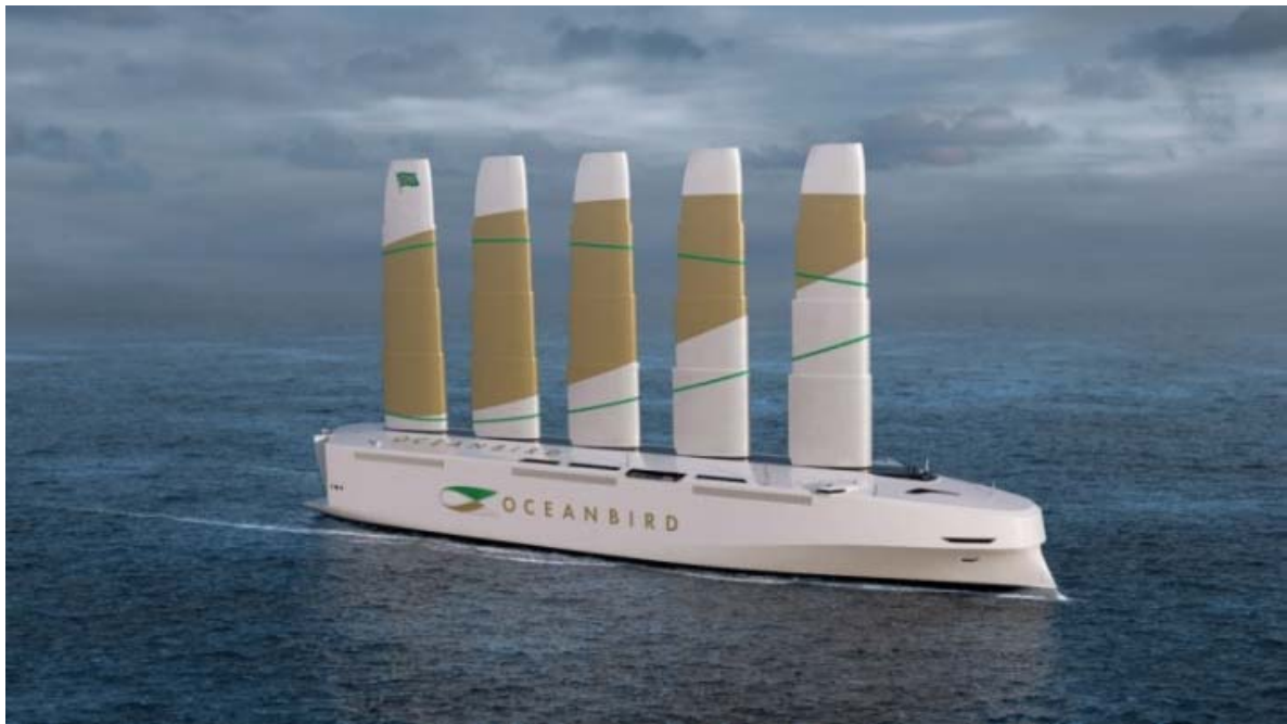
Figure 3 – Example of implementation investment project “Utilizing windsails to decrease fuel consumption”
