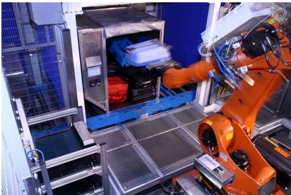
Pic.2. Robot loading luggage into a container.
